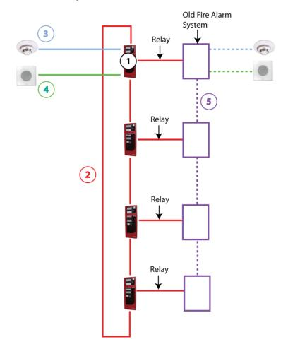
4. Transferred full audio capabilities from the existing system over to the FleX-Net MNS transponder units
