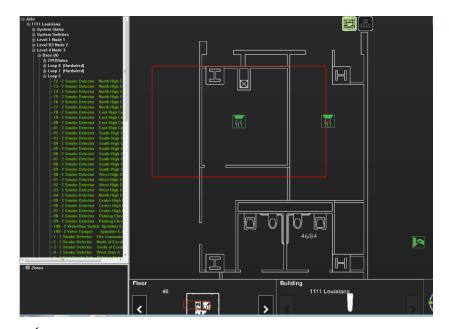
A dedicated PC terminal to operate the Open GN application was mounted within the BB-5008 Fire Alarm Control panel with a custom fitted 24" Touchscreen.
