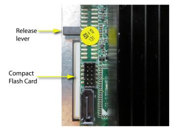
2. Insert the new card into the slot.
