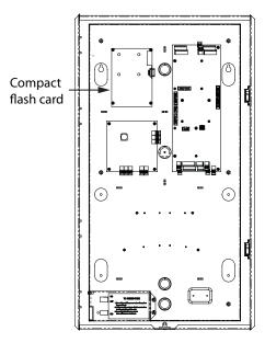
1. Press the black release lever to eject the compact flash card.
