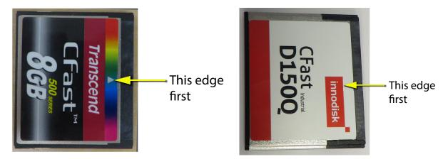
The card should slide in easily and rest in the same location as the old card. Forcing the card can damage the equipment.
