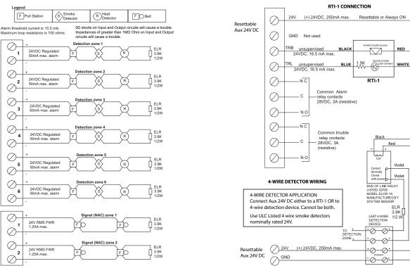
\*The FA-103 has the same features as the FA-106 except there are three detections zones and not six. The enclosures and boards are identical. The FA-103 is depopulated and has terminal connections for three detection zone.
