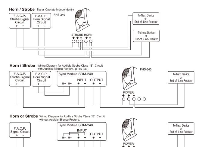
Refer to the SDM-240 Sync Module instruction manual for Class "A" wiring or other application diagrams.
