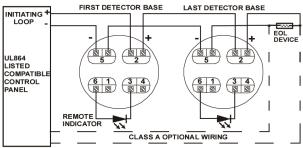
NOTE: IF REMOTE INDICATOR IS NOT USED, REVERSING POLARITY ON DETECTOR IS PERMITTED.
