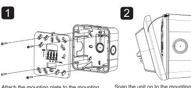
Attach the mounting plate to the mounting box with the 4 screws.
