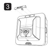
Secure the unit with the #4-40 x 3/8" screw and snap the nameplate over the screw.
