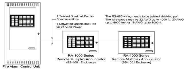
NOTE: Annunciator wiring must be as shown. Star type or 'T' tap connections are not allowed. The RA-1000 Series Remote Annunciators must be wired in a loop configuration.
