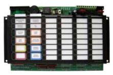
The RAM-1032TZDS Main Remote LED Annunciator provides common annunciator functions and 32 points of LED annunciation. The RAM-1032TZDS has indicators for A.C. On, Common Trouble and Signal Silence and controls for System Reset, Lamp Test, Fire Drill, Buzzer Silence and Signal Silence. The RAM-1032TZDS occupies one display position in the BB-1000 or BB-5000 enclosures.
