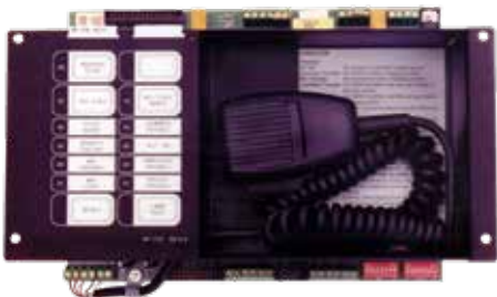
QMP-5101N Network Master Paging Control Module The QMP-5101N Network Master Paging Control Module includes the paging microphone and common control indicators. The QMP-5101N allows for all call paging or selective paging with the QAZT-5302DS Zoned Paging and Telephone Selector Modules. The QMP-5101N occupies one module space in the BB-5000 Series enclosures.
