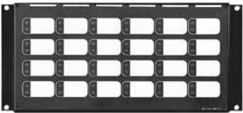
QAZT-5302DS Zoned Paging and Telephone Selector Module The QAZT-5302DS Zoned Paging and Telephone Selector Module includes 24 zone selector switches and LEDs. The QAZT-5302DS is used with the QMP-5101N Network Master Paging Control module or QMT-5302N Network Master Firefighters' Telephone module. Slide-in labels are provided to label the selector zones. The QAZT-5302DS occupies one module space in the BB-1000 or BB-5000 Series enclosures.
