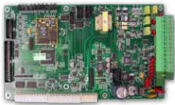
ANC-5000 Audio Network Controller Module The ANC-5000 provides audio microphone control on the network system. The ANC-5000 mounts on a plate in the QMB-5000N.
