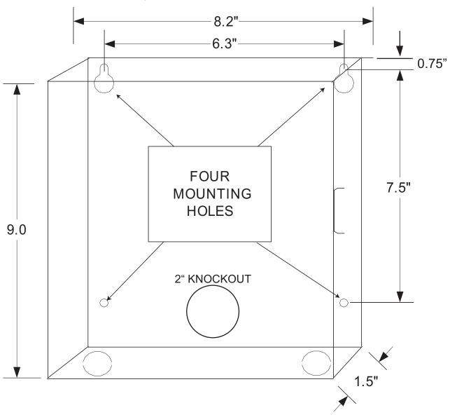
Figure 1 SRM-312 Mounting Dimensions
