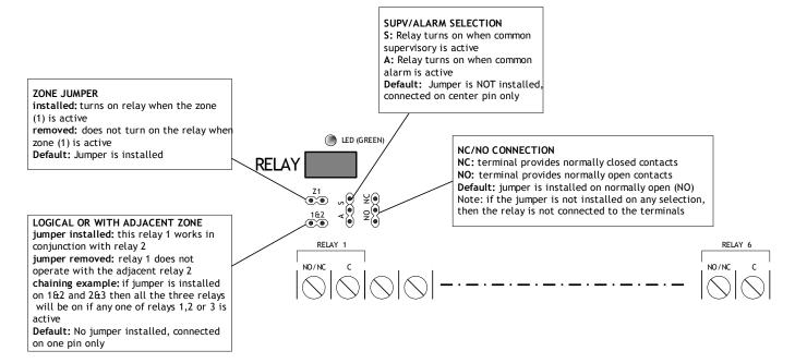
Figure 3 Relay Configuration
