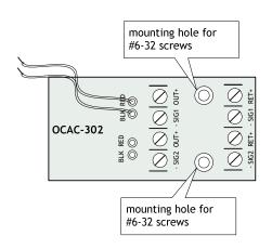
Indicating circuits must be wired from the OCAC-304/302 to the main Fire Alarm board. For example indicating circuit 1 positive (red wire) and negative (black wire) is wired from the Class A converter module to the positive and negative terminals of Indicating circuit 1 on the Main Fire Alarm board.
