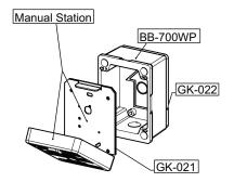
7. Ensure that the arrow on the inside of the BB-700WP is pointing upwards and unlock the manual station.
