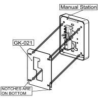
5. Align with the four mounting holes and terminal block on the back of the manual station.
