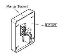
6. Press the adhesive side of the GK-021 firmly into place on the manual station.
