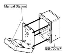
8. Align the four mounting holes of the manual station and the BB-700WP.
