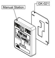
4. Remove the adhesive backing paper from the GK-021 neoprene gasket.
