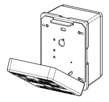
9. Firmly press the manual station onto the BB-700WP and secure with the screws provided.
