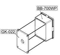
2. Align the four screw holes on the back in the gasket with the matching holes on the back of the BB-700WP.
