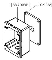
1. Remove the adhesive backing paper from the GK-022 neoprene gasket.
