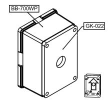
3. Press the adhesive side of the GK-022 firmly into place on the BB-700WP. The BB-700WP is now ready for mounting. When mounting the BB-700WP ensure the arrow on the inside of the backbox is pointing upwards.
