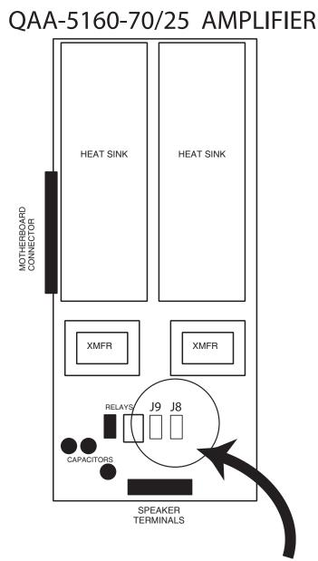
FOR AMPLIFIER TO OPERATE AS 25V, REMOVE ORANGE CABLE LABELLED MD-790 FROM J9 AND J8 AND REPLACE WITH BLUE CABLE MARKED MD-791 BETWEEN J9 AND J8.
