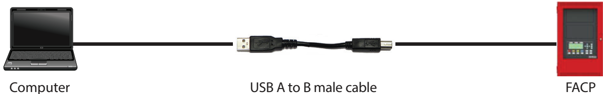
Figure 7 USB A to B male cable to P13 on main board
