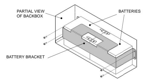
Place the bracket over the batteries as shown in the figure above.
