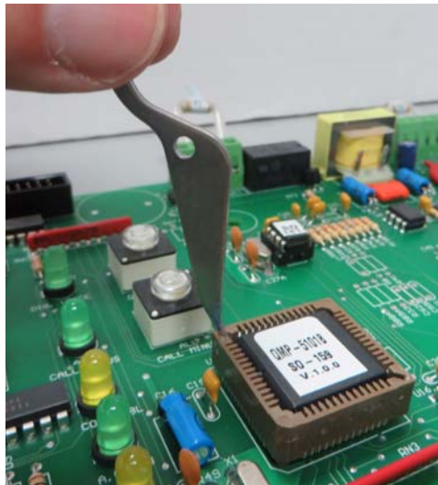
Figure 2 The extraction tool inserted into the socket
