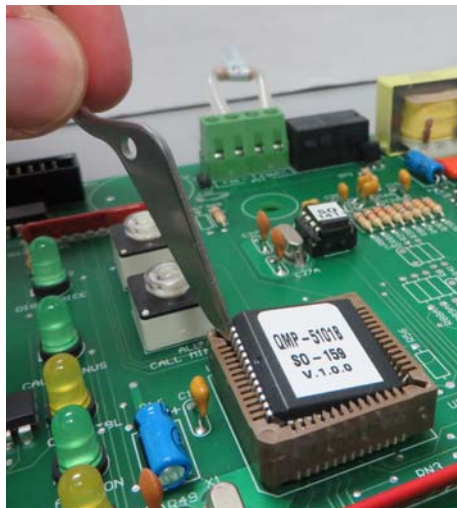
Figure 3 The extraction tool lifting the chip out of the socket
