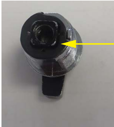
Figure 3 Stop cam washer with the gap on the upper right
