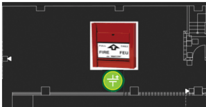
Figure 7 A floor plan showing an imported image above a device icon
