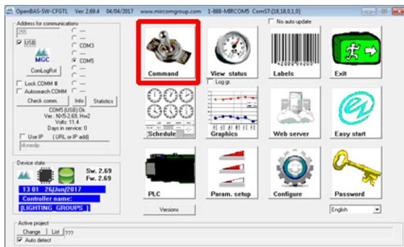
16. The command window allows the user to view all the values and states of the analog inputs and binary outputs. As shown below, analog input 3 is greater than input 2 and thus the second lighting group (outputs 5-8) is on.
