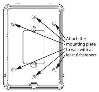
Use 2 screws to align gang box with mounting plate
