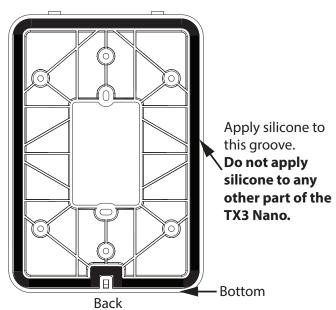
Attach TX3 Nano to mounting plate
