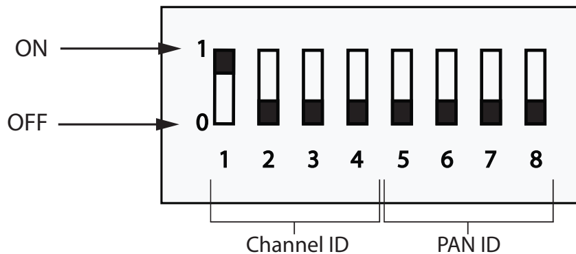
Figure 7 DIP Switches on the Zone Controller set to Channel ID 19 and PAN ID 1126
