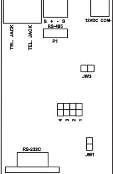
LT-634 Rev.5 January 2007 **MOUNTING THE MODEM INTO THE MUS-5000 OR MCS-6000** - use the double-sided tape to mount the MODEM across the top of the backbox above the main board.
