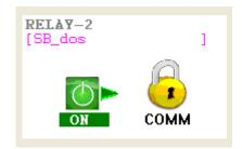
If there is a **LOCAL OVERRIDE**, the command buttons ON/OFF and of OVERRIDE COMM and RELEASE will be disabled. The only way of liberate them will be locally in the LCD operator display.
