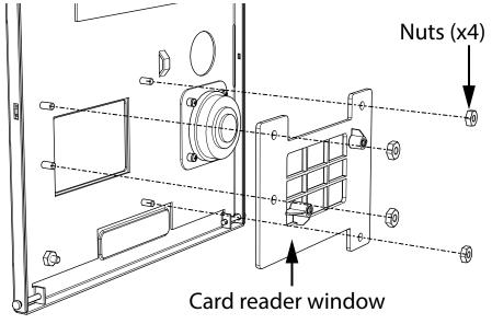
3. Use the 4 Nuts to Secure the Postal Lock Window, Plate, and Switch Holder
