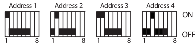
Figure 5. Setting the RS-485 address
