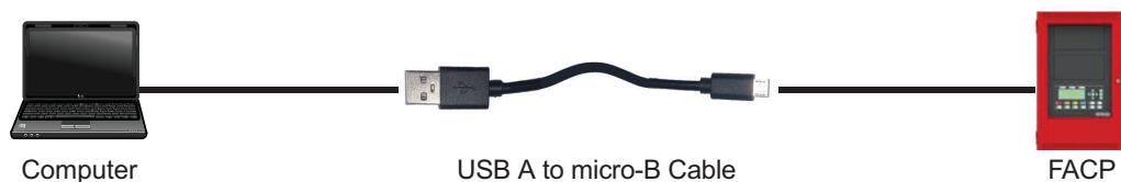
Figure 22 USB A to micro-B plug cable to P5 on core board
