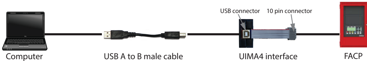
Figure 23 UIMA4 to P5 on main board
