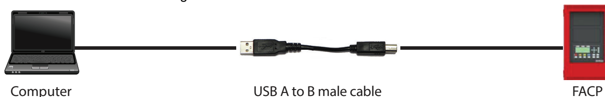
Figure 22 USB A to B plug cable to P13 on main board
