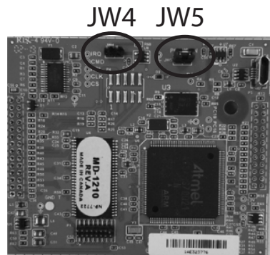
Figure 88 Jumpers on the FX-400 and FX-401 core board
