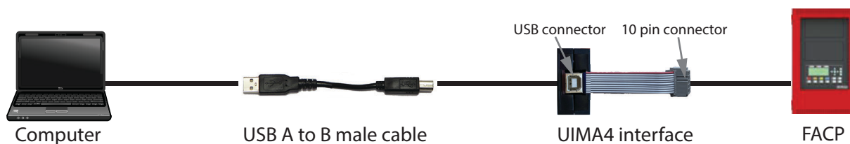
Figure 23 UIMA4 to P5 on main board
