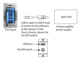
If the USB A male to B male cable is too short, use an Ethernet cable (not included) and the included USB over Ethernet extender cables as shown below. The maximum distance is 46 m (150 feet).
