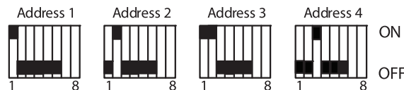
Figure 2 Set the RS-485 address
