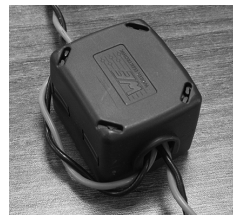
Ferrites installed on the power cable and Ethernet cable in a 4x4" electrical box with a depth of at least 2.7"
