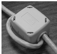
Ferrites installed on the power cable and Ethernet cable in a 4x4" electrical box with a depth of at least 2.7"
