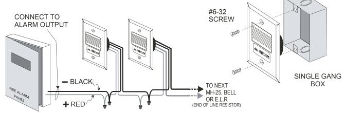
Use both leads for connection. Break wire run to provide electrical supervision.
