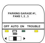
AUTO LED shows steady for switch in AUTO position.
