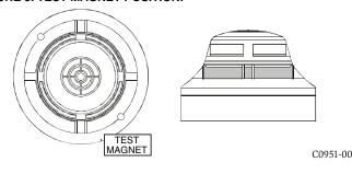
For MIX-COSAP, smoke entry testing should be performed immediately following the magnet test. Magnet test initiates an approximately 10 minute period when the detector's signal processing software routines are not active. Failure to first perform the magnet test will introduce a time delay before the detector alarms.
